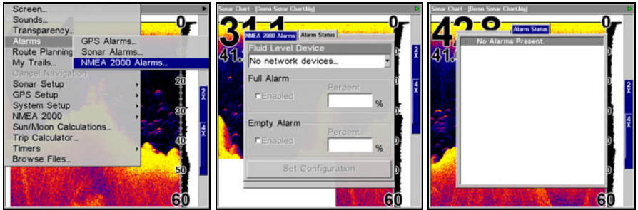
NMEA 2000 Alarms highlighted on Alarms menu (left). NMEA 2000 Alarms menu (center). Alarm Status page (right).
